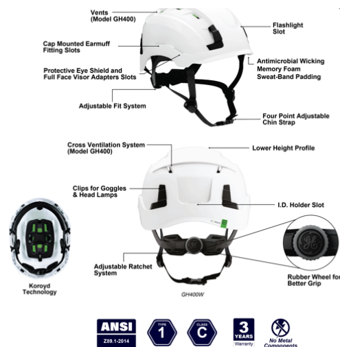
Figure 2: Key features of the GH400 Safety Helmet.
