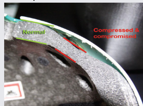
Compromised EPS under the shell
