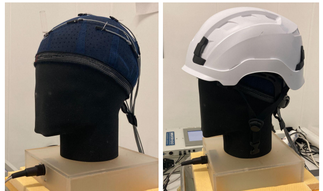
Figure 2: Laboratory test setup of the Sweator Head
